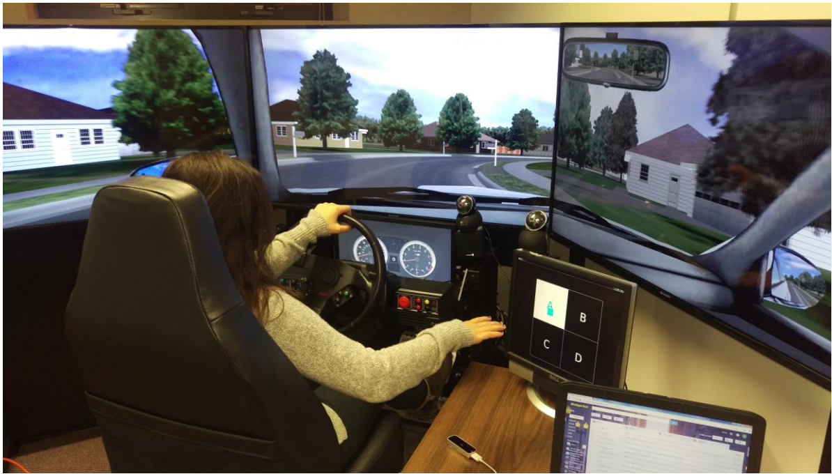
Figure 3: Driving simulator setup, visual display monitor with webcam, LEAP Motion.
